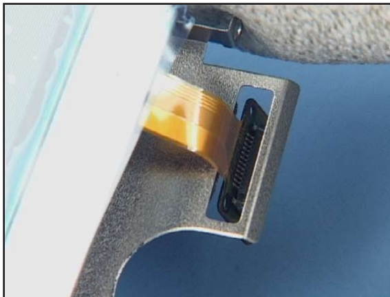
20. Slot through the flex foil of the LCD MODULE.
