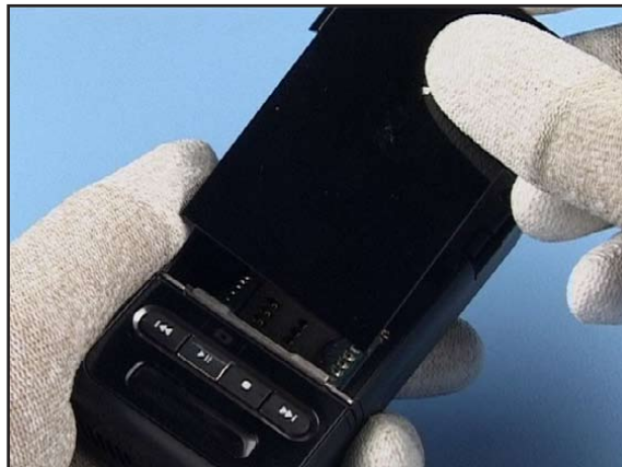
32. Complete the assembly by placing the BATTERY COVER.
