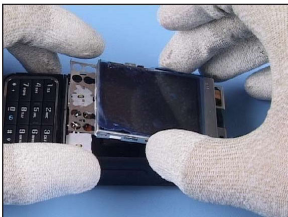
23. Flip over the DISPLAY SHIELD ASSEMBLY and push it into its place.
