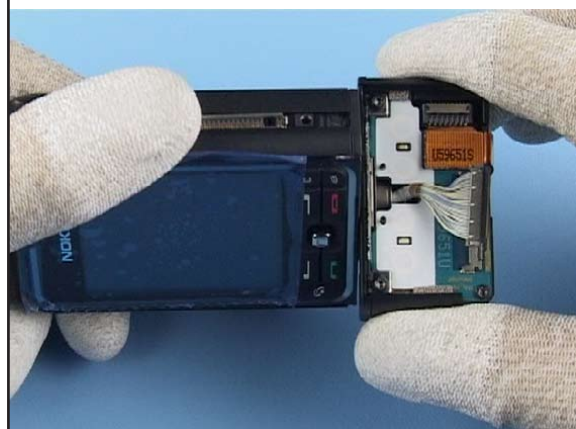
6. Turn the unit to prevent mechanical stress to the joystick.
