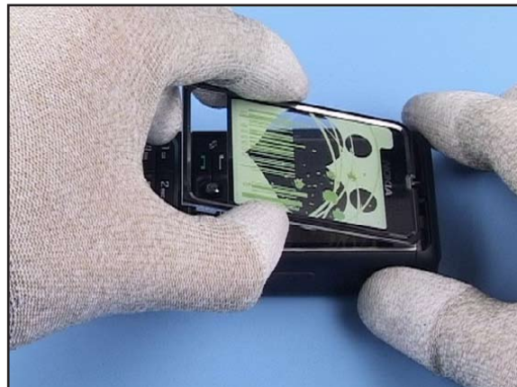
30. Remove the cover tape and place the new A-COVER ASSEMBLY, beginning from the top.
