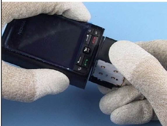
11. Turn the upper block in order to prevent mechanical stress to the joystick while unscrewing the screws.
