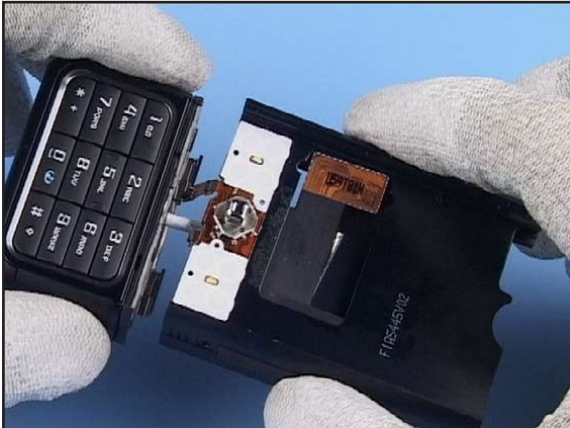
7. Bring the Lower Block into position above the UPPER FRAME ALUMINIUM and align the 2 SWIVEL SENSORS into their guides.
