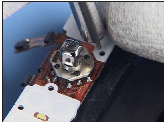
4. Align the DOMESHEET with the SIM Tool, mind the surrounding components.
