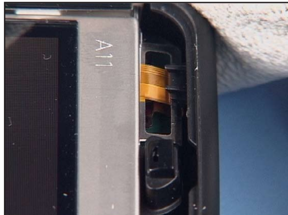
28. Place the CAP COVER and fix both latches.
