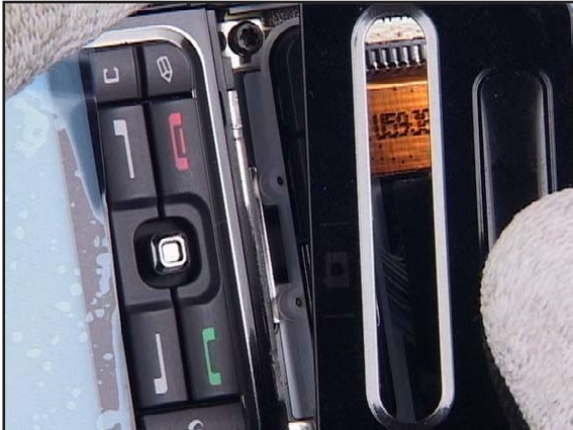
7. Turn the assembly and remove the LOWER BACK COVER.
