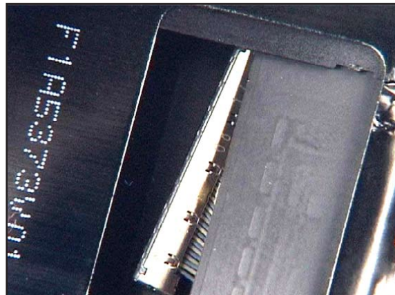
24. Carefully separate the lower block, but remember the UPPER BLOCK CONNECTOR.
