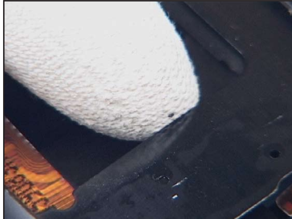
26. Push down the MAIN FLEX ASSEMBLY with your thumb to release the adhesive tape from the UPPER FRAME ALUMINIUM.
