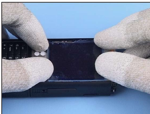
24. Fix it using finger pressure.
